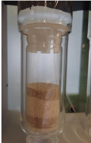
Figure 1: Twisselmann extraction chamber before start
